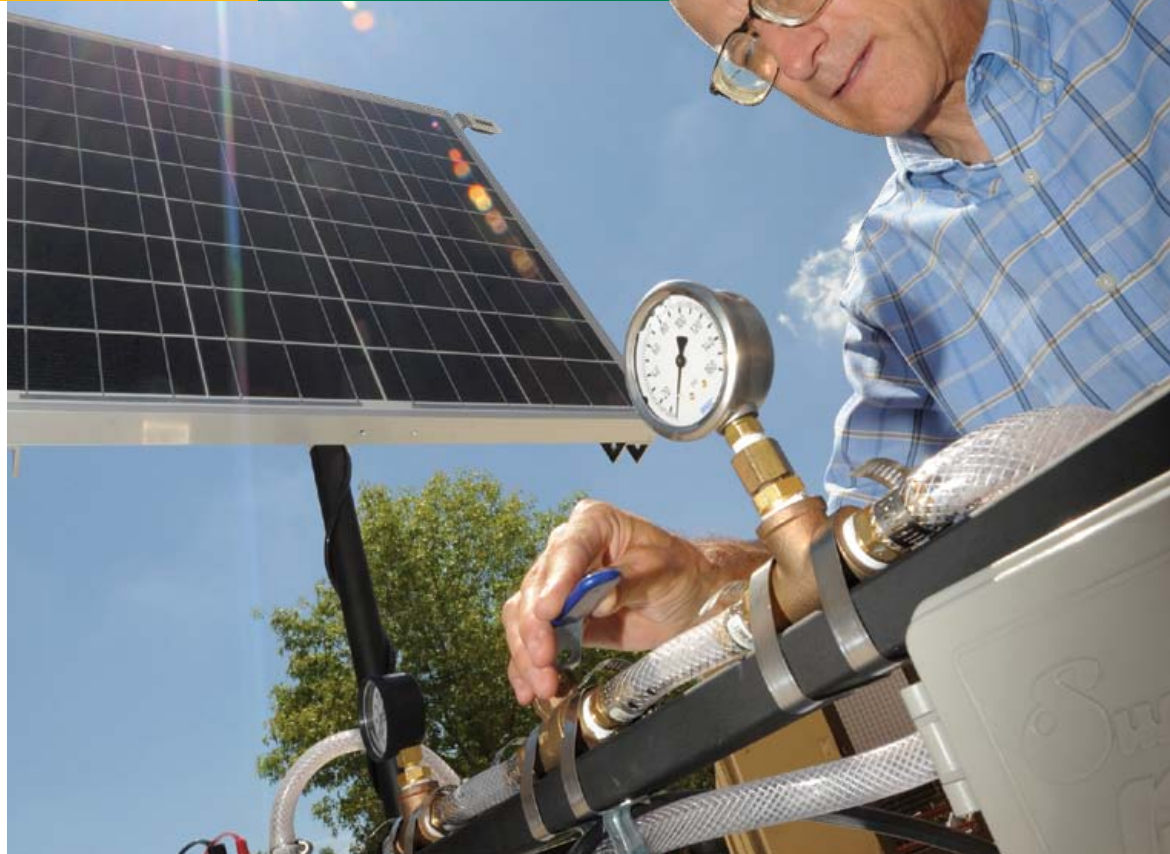
Associate professor Craig Ricketts supervised the work of three mechanical engineering technology seniors who designed and built a solar-powered water pump for Cooperative Extension Service agents to use for field demonstrations.
